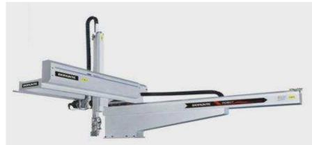
BRR Series is applicable to all types of horizontal injection machine ranges of 30~320T for take-out products and sprues. Vertical arm is single stage. With types of three-axis and five-axis driven by AC servo motor. Products take-out at super high-speed (0.8sec) and dry cycle time within 5 seconds, applicable to take-out products with the function of mold labeling and mold inserting.
